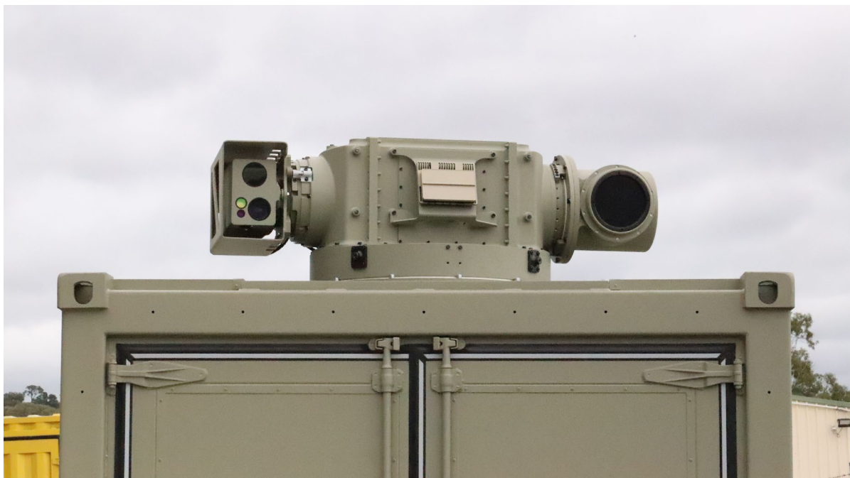
Figure 1: An operational DE beam director installed on a standard 20' container
